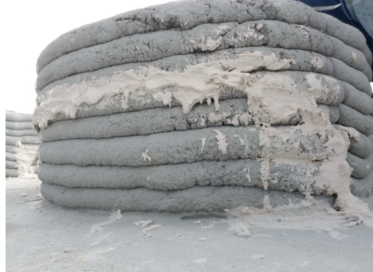
b) Ceramic adhesive fiber attachment
