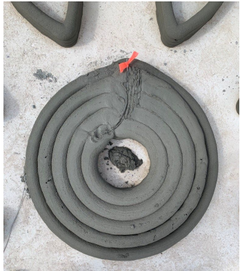
a) Thermocouple embedding
