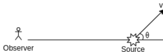
Figure 8: Doppler shift for a moving source
