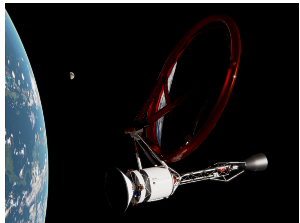
Figure 2: Conceptual render of a Laser-Thermal-Propulsion System, carrying a 1 ton payload for a 45-day Mars transfer
