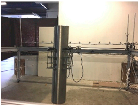
Fig. 22. PoC Smart Catcher on Themis alternative landing system.
