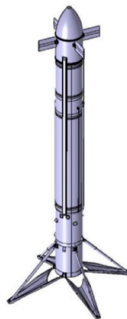
Fig. 13. CALLISTO Vehicle configuration fins and legs unfolded.
