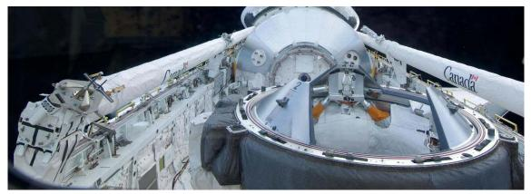
Figure 4: The mounted ODS as seen looking through the space shuttle cargo bay windows
