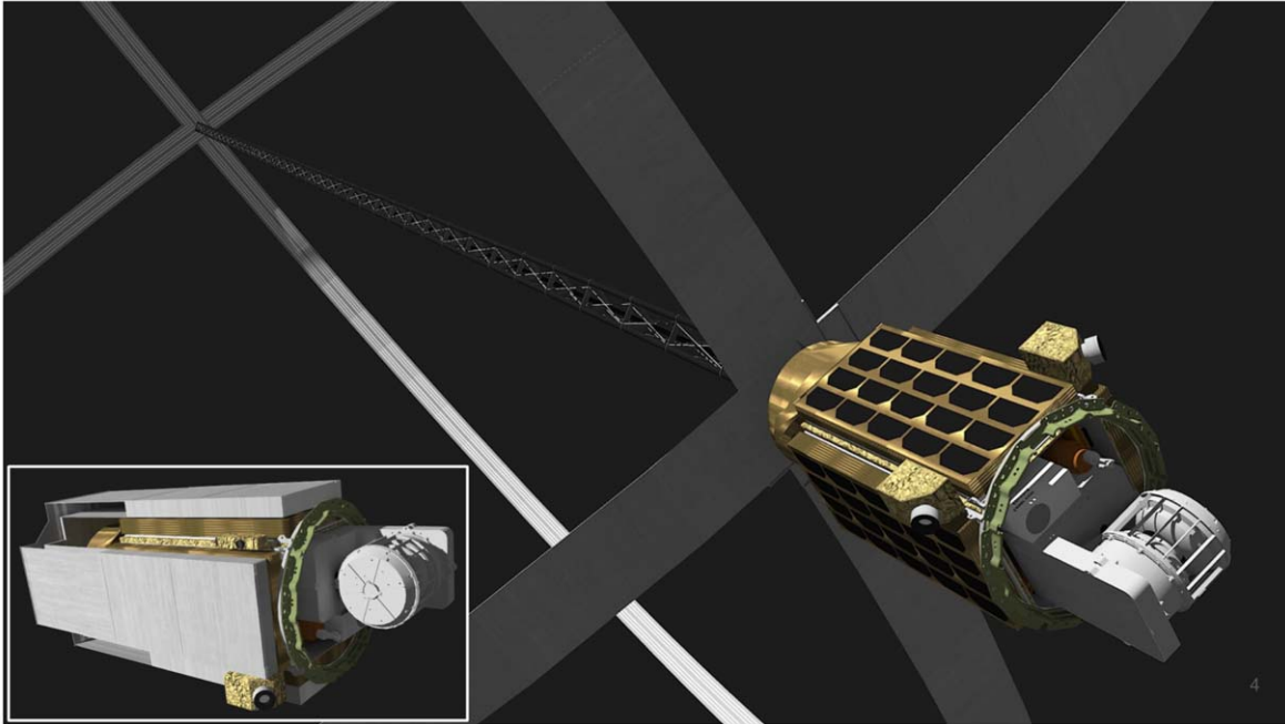
Figure 2. JOVE model pre- and post-deployment of the HTS coils. The mast is 9 m long.
