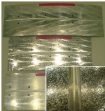
Figure 18. Meridional R = 3000 mm (dome, C-FSW), Longitudinal/axial (cylinder, C-FSW) (Material from forming demonstrators)
