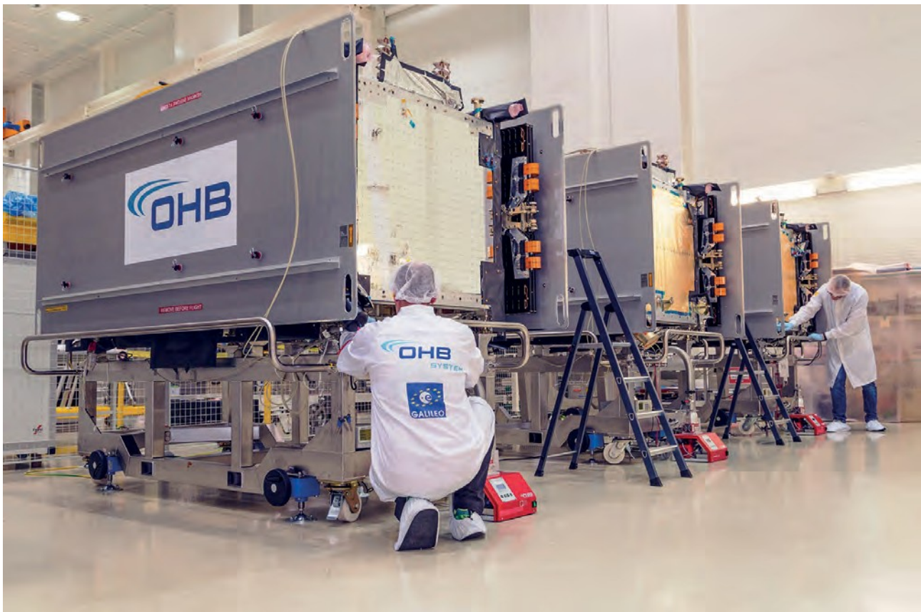
Photo 1: Serial integration of Galileo satellites.
