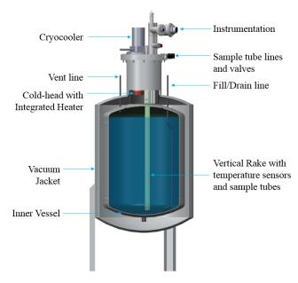
Figure 3. Cutaway view of LNG cryostat apparatus.
