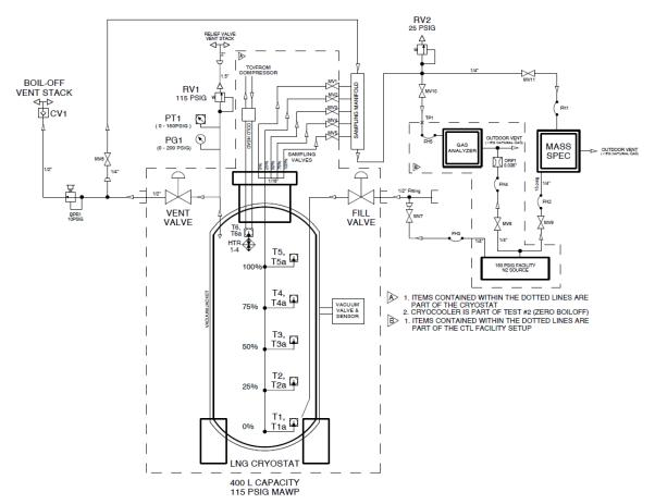
Figure 2. Test schematic of LNG cryostat apparatus.
