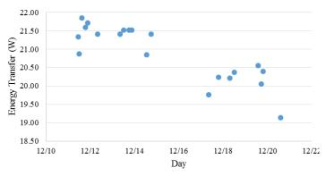
Figure 4. Heat leak of cryostat from the LN<sub>2</sub> boiloff test.
