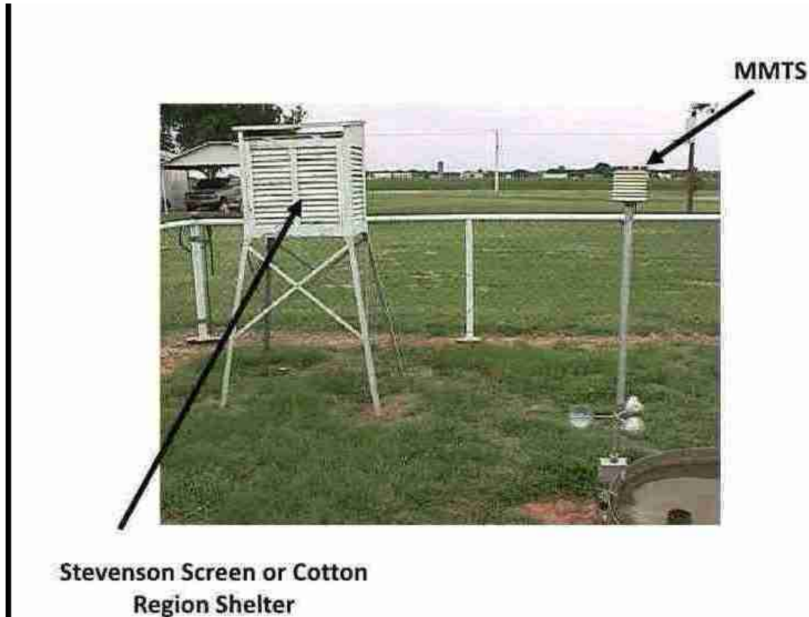
Figure 2: Examples of Stevenson Screen aka Cotton Region Shelter enclosures (left) and the newer MMTS electronic sensor enclosure (right). Source: Pat Guinan. 7
