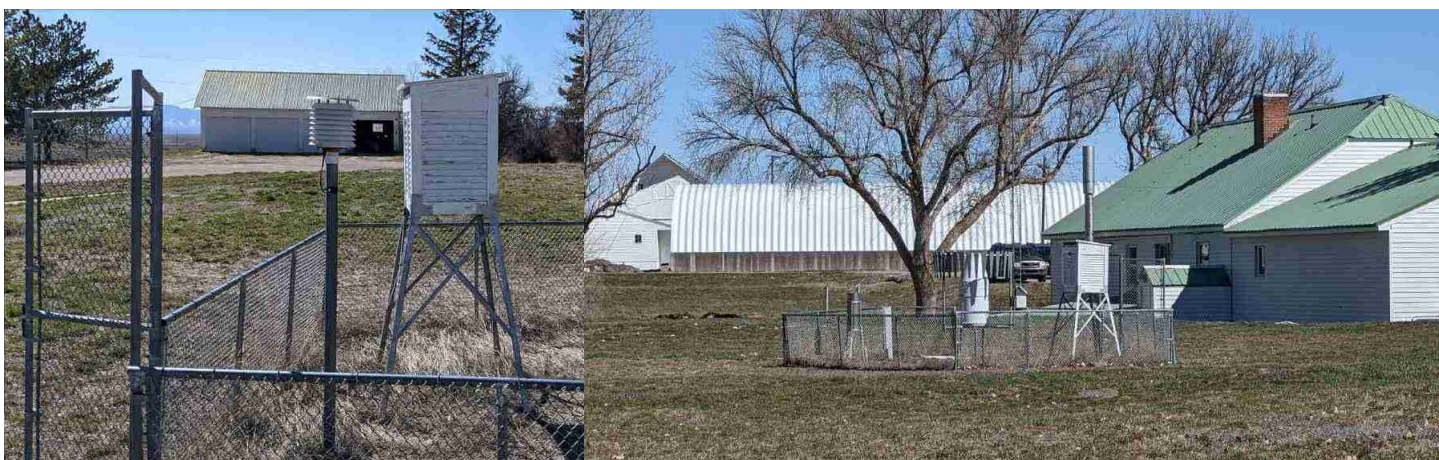
MMTS and CRS placement in a large grass field at USDA Agricultural Research Farm in Dubois, ID. This station is properly sited, and is one of two Class 1 rated stations located in the 2022 survey. Source: Anthony Watts.
