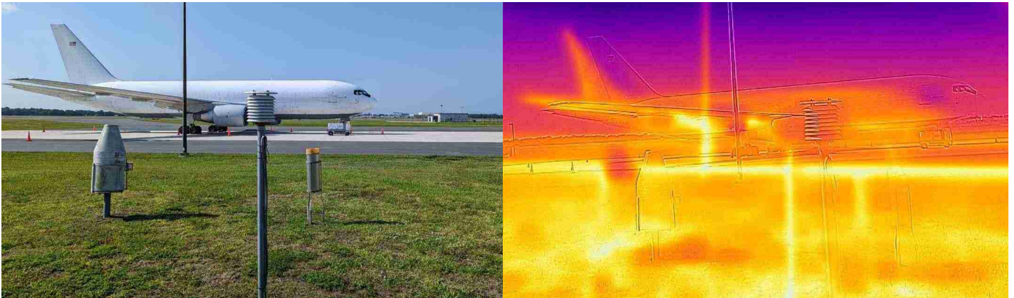
Visible and infrared photos of MMTS placement near airport ramp tarmac at GHCN station in Lakeland, FL. Source: Anthony Watts.
