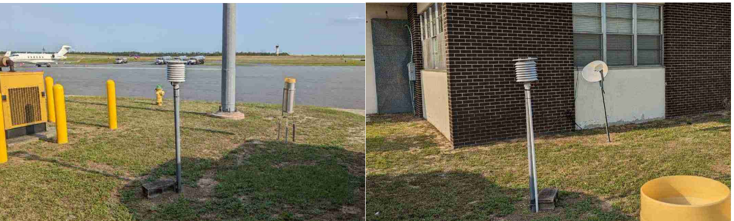
MMTS placement at the airport fire station in Tallahassee, FL, a GHCN station. Note the proximity of multiple heat sources and sinks. Source: Anthony Watts.
