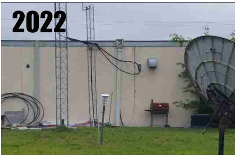
No change in location, but MMTS is now tilting due to lack of maintenance. RATING = CRN4
