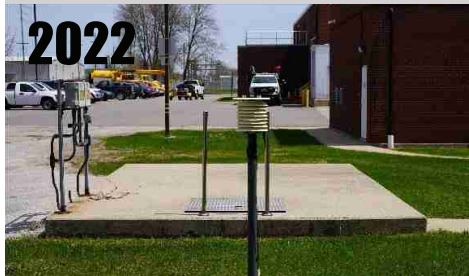
Same location at WWTP, but moved and converted to MMTS. Slightly better siting compared to original location. RATING = CRN4
