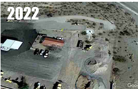
Same location, but CRS updated to MMTS. Still close to building and asphalt parking lot. RATING = CRN4
