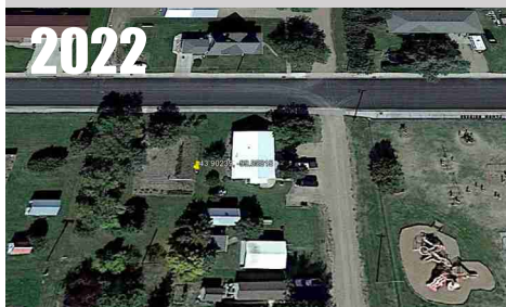
Same location, but NWS reports: "moved MMTS 35 feet to the northwest due to bad location." Unable to ground survey. RATING = CRN4
