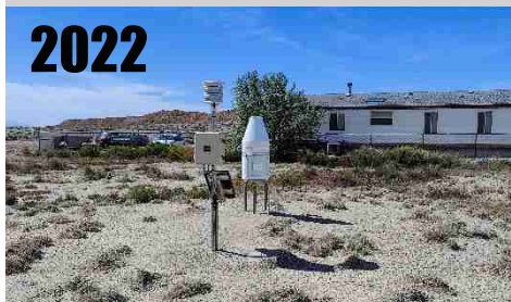
Site moved, new wireless MMTS provided. Better location. NWS reports: "SITE MOVED 1.99 MILES EAST SOUTHEAST" RATING = CRN2
