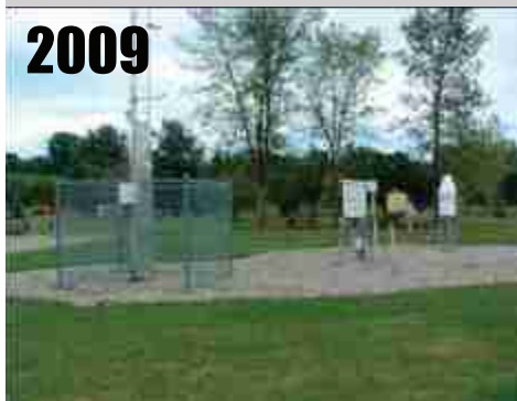
Sandpoint, ID , heavy gravel base, near road. RATING = CRN4
