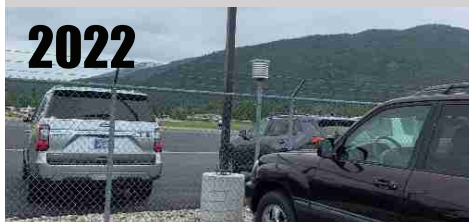
MMTS was relocated to even worse site 0.31 miles away to the airport parking lot, sandwiched between airport tarmac and airport parking. Note vehicle radiator is directly under the sensor. RATING = CRN5
