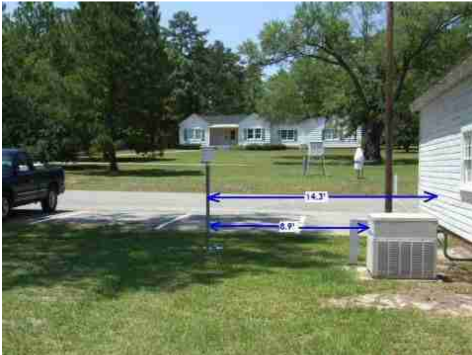
Figure 4: Old Stevenson Screen / CRS and new MMTS / Nimbus electronic thermometer in Bainbridge, GA, circa 2008. The new MMTS station moved about 150 feet closer to the building to accommodate the new MMTS sensor cable length. The MMTS is recording heat from the air conditioning unit exhaust, house, cars, and asphalt parking lot, whereas the original placement had none of these issues. The station has since been closed by NOAA / NWS. Source: Joel McDade.
