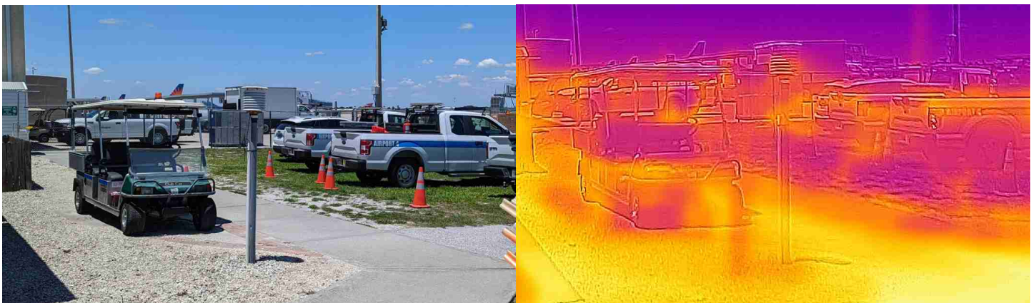
Visible and infrared photos of GHCN station located at the FBO office at Punta Gorda Airport, FL. The station is surrounded by heat sinks. Source: Anthony Watts.
