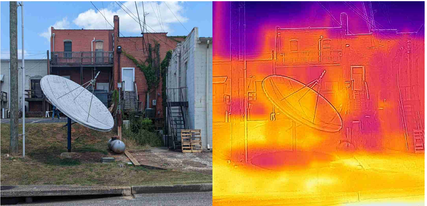
Visible and infrared photos of USHCN station in Troy, AL, at a radio station parking lot. Multiple heat sinks and sources are visible within feet of the sensor, including a/c units, asphalt, and concrete. The MMTS is mounted on top of a brick retaining wall. Previously, it was placed in the grass near the satellite dish. Source: Anthony Watts.
