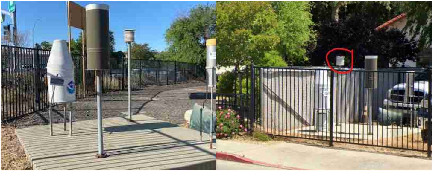
USHCN station at Paso Robles, CA, on Paso Robles Boulevard. Note it is located between U.S. Route 101 and is directly over a concrete slab. This is a Class 5 station that is saturated with heat sinks. Source: Dacre Bush / Google Earth Street View.
