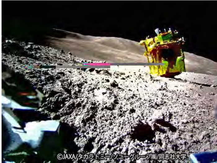
Image from Lunar Exploration Vehicle (LEV-2) of Japan's lunar lander. SLIM Vehicle is missing one rocket nozzle and is on its nose. (@AndySaunders_1 & @JAXA_en via X)
