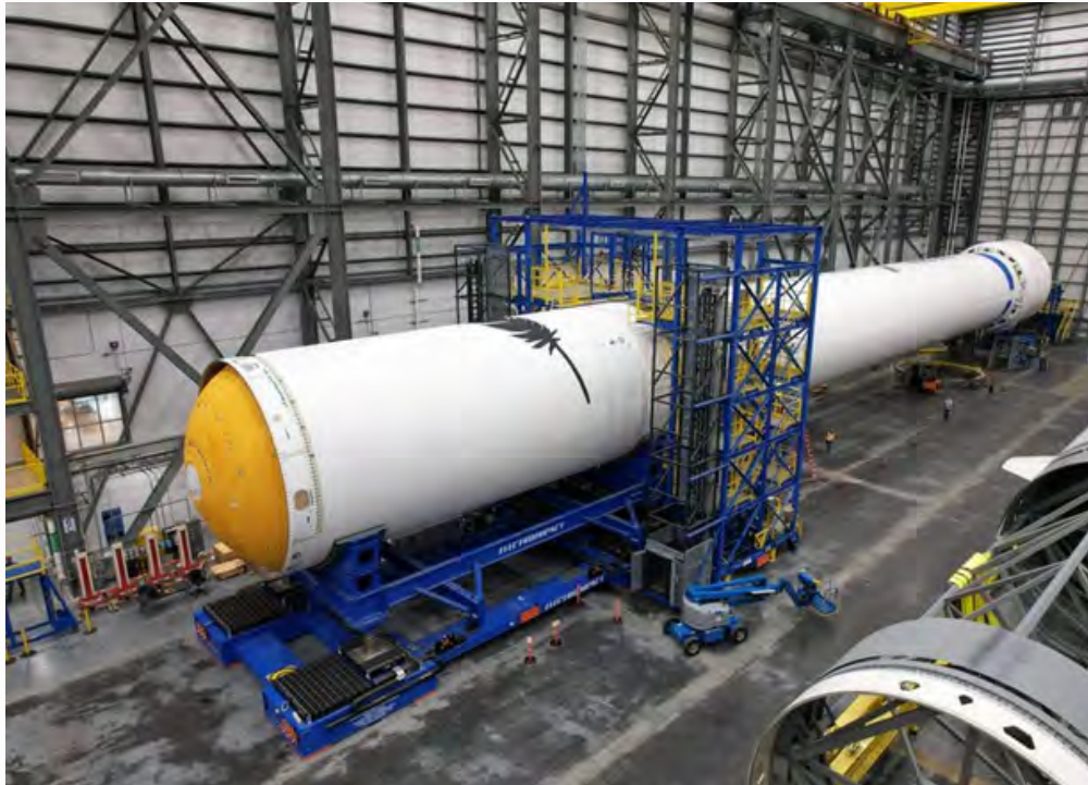
Blue Origin's New Glenn 1st and 2nd Stages Mate for First Time. First launch expected later in 2024. Estimated capacity: 50T to LEO ( @blueorigin via X)
