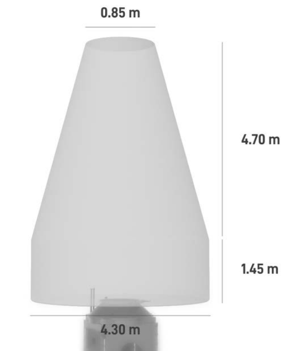
Figure 4-1: Cake Topper Payload Keep-In Volume
