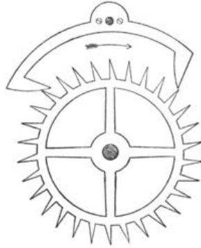
Figure 15: Simple example of a clock escapement
