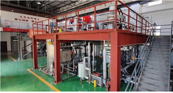
图 11 (网络版彩图) 锂冷空间堆系统集成原理实验样机 Figure 11 (Color online) Integrated experimental of lithium-cooled space nuclear reactor.
