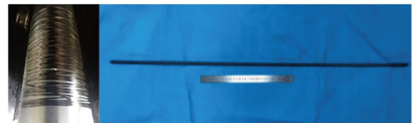
图 9 (网络版彩图)金属内衬SiC f /SiC复合材料薄壁管样件 Figure 9 (Color online) Metal lined SiC f /SiC composite thin-walled pipe sample.
