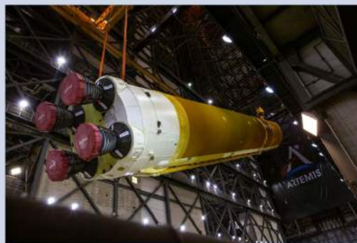
The SLS core stage being raised in the Vehicle Assembly Building for stacking of the Artemis I rocket.
